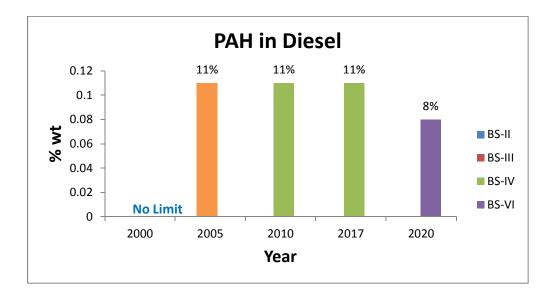
Criterion for limiting PAH was for the first time introduced for BS-III diesel as 11% wt. max and has further been reduced to 8% in BS-VI specification in line with Euro-VI norms.
